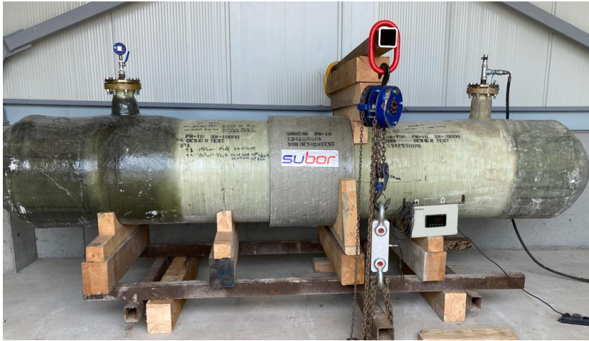
Photos 2 : Deformation with internal / cyclic pressure and end thrust
