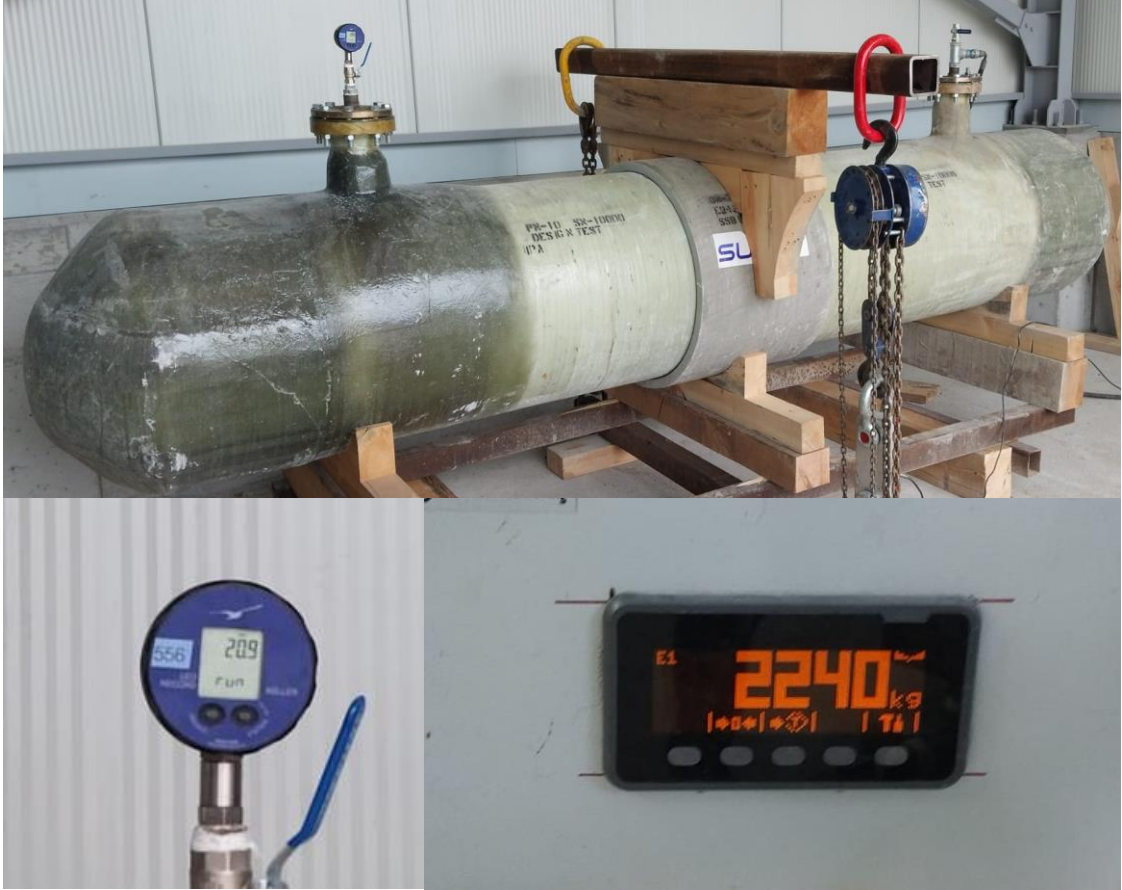
Photos 3 : Method A Resistance to bending with pressure and end thrust
