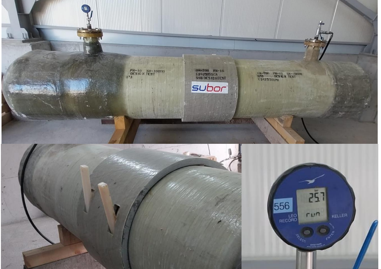
Photos 4 : Resistance to maintained internal pressure and end thrust
