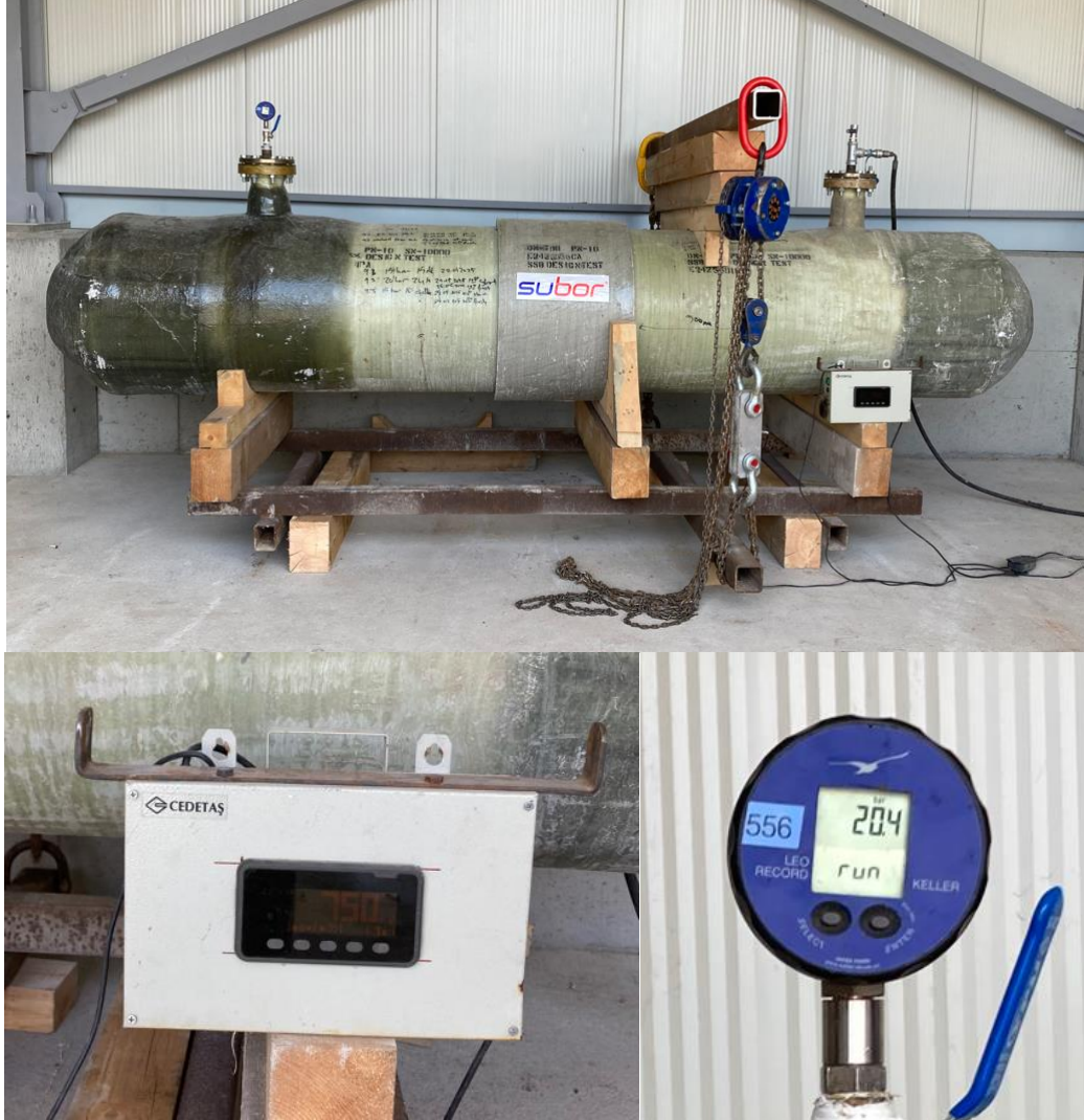
Photos 5 : Hydrostatic Test in Shear Loading Position
