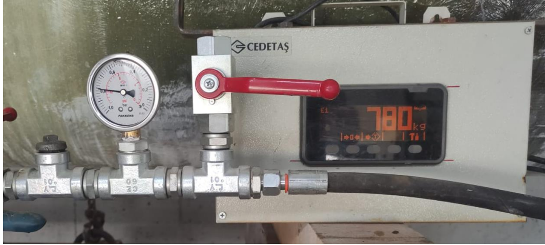
Photos 6 : External Pressure Test
