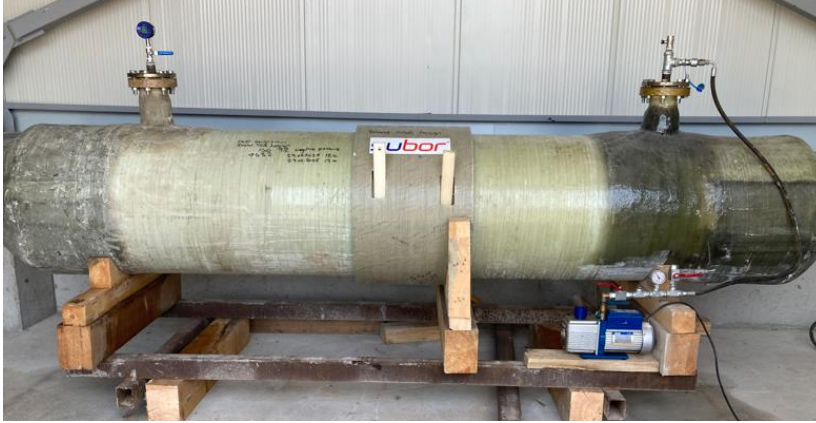
Photos 1 : Negative pressure test
